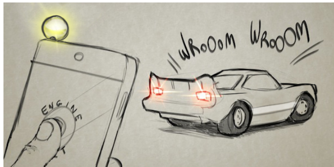
Fig. 1. (© Disney) VLC enabled toy remotely controlled by a smartphone extension device plugged into the audio jack.
