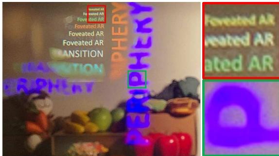
Fig. 17. Display photographed through the display of the wearable prototype. The top, red inset shows a detail from the foveal region and the lower, green inset is from the peripheral region. Note that the smaller projector used in the wearable prototype has narrower light cone angle and worse color representation which led to smaller FOV ( 77^\circ \times 53^\circ ) and severe color mismatch.
