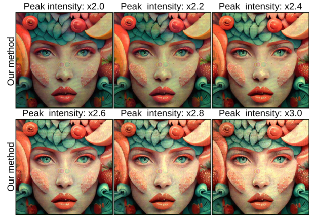
Figure 3: Increasing peak intensity levels with our multi-color hologram scheme. Photographs show that our method can enhance the peak intensity levels of the captures up to \times 1.8 without noticeable artifacts or distortions. In contrast, the conventional hologram fails to support beyond \times 1.0 (Source image: Midjourney, Link: Github:complight/image, 140 ms exposure).
