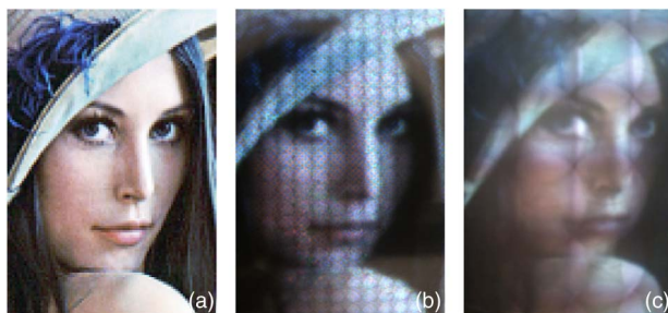
Fig. 7. Picture and two photographs showing (a) desired target image, (b) image observed through an HMD prototype with overlap ratio of 76% between retinal elemental images, and (c) image observed through another HMD prototype with a lower overlap of 30%.
